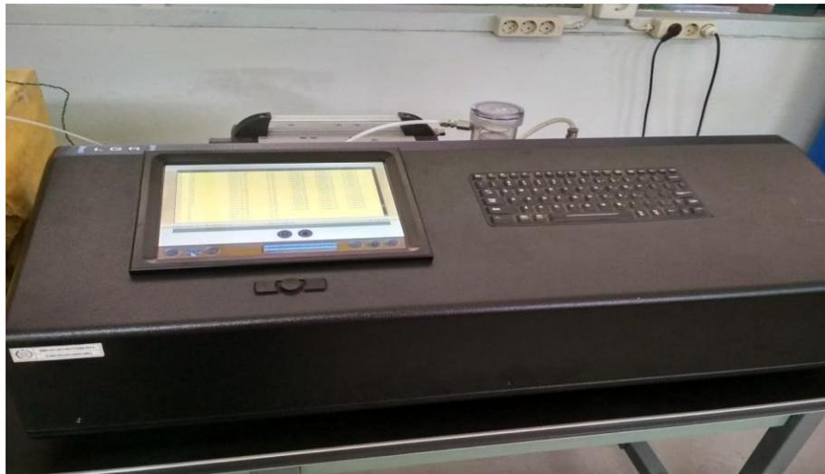
**Gambar 3.4.** Perangkat LGR(*Los Gatos Research*) DLT-100 *liquid water stable isotope analyzer*
