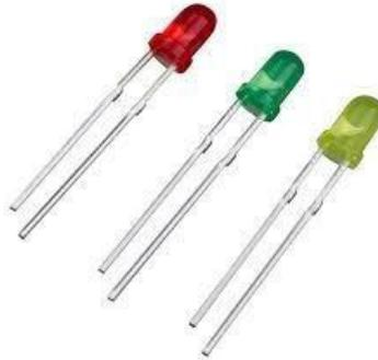
Gambar 2.7 *Light Emitting Diode (LED)*
